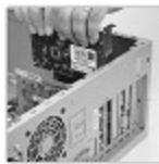
Figure 3 Use firm pressures to push the card into the slot—and make sure that the card is firmly seated.
